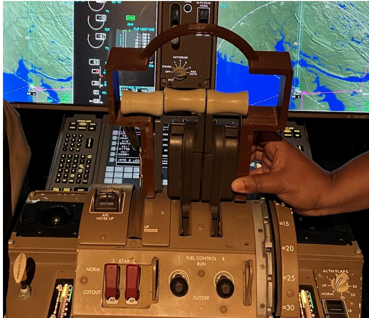
Fig. 3 The three throttle concept in the RFD. Throttles #1 (left lever) and #3 (right lever) were physically linked and controlled the electric engines. Throttle #2 (middle lever) controlled the turbine engine. The physical link was installed only for the 3 throttle concept (Photo Credit NASA).
