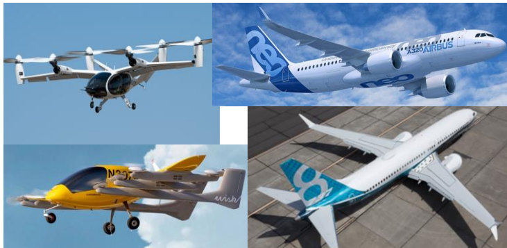
Figure 1. Examples of single-aisle and all-electric transports. Clockwise from top right: Airbus A320neo, Boeing 737 MAX, Wisk Aero Cora, and Joby Aviation S4
