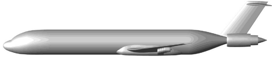
Fig. 6. SUSAN 25%-scale concept fuselage structure.
