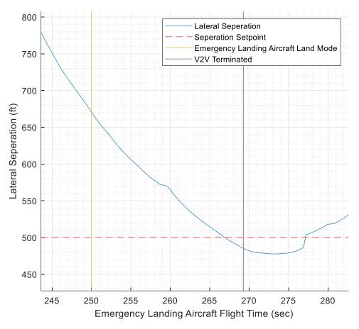
Figure 52: Lateral Separation Plot of Test Run 3 ATAM on April 26th
