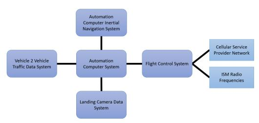
Figure 2: Aircraft Systems High Level Diagram
