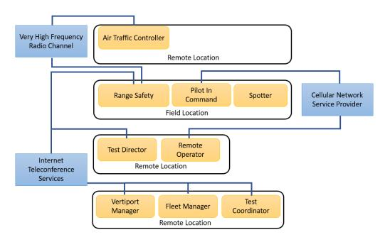
Figure 13: Voice Communications System Diagram
