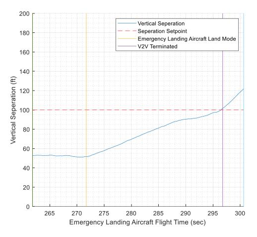
Figure 33: Vertical Separation Plot during Test Run 3 ATAM on April 12th
