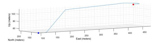
Figure 46: 3D Vertical Profile Plot of Test Run 4 AELM on April 21st
