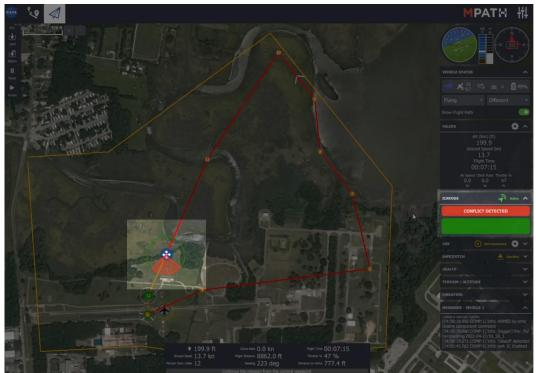
Figure 24: ATAM Display on the remote GCS in ROAM
