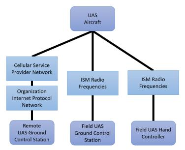
Figure 10: High Level C2 System Diagram
