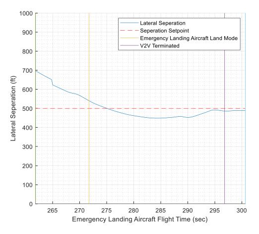
Figure 34: Lateral Separation Plot during Test Run 3 ATAM on April 12th
