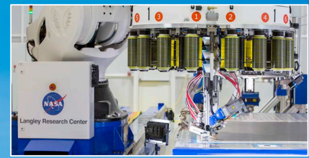
High-Rate Composite Manufacturing 4-6x manufacturing rate increase
