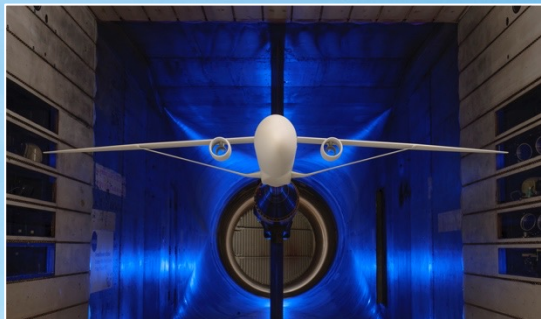
Transonic Truss-Braced Wing 5-10% fuel burn benefit
