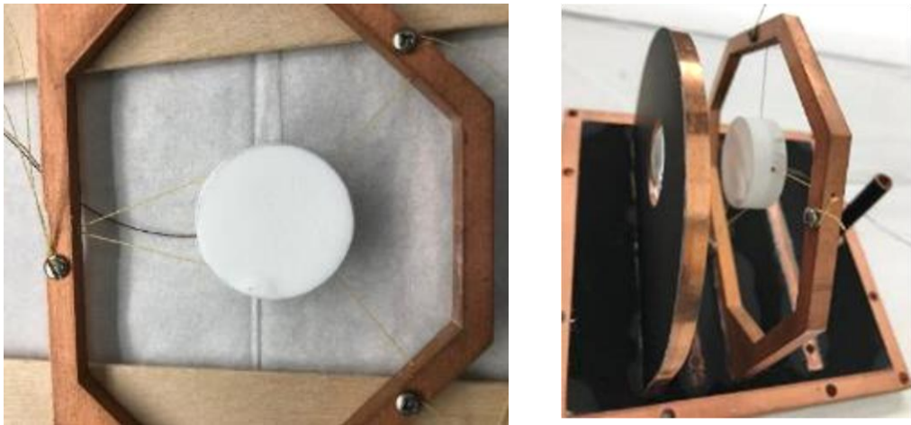
Figure 3-18. Images of the AZ-93 sample mounted in a frame using Kevlar string, ready to be lowered into the test enclosure.
