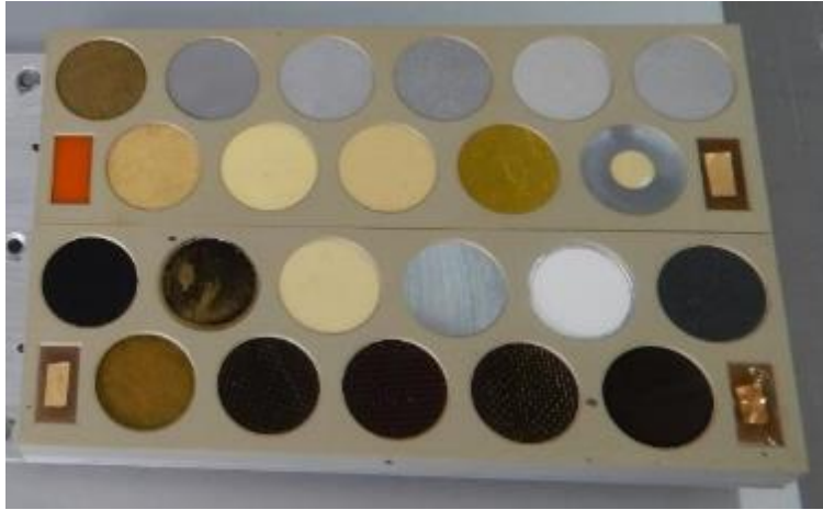
Figure 3-29. MISSE-11 tray containing the Y_2O_3 tile (white tile).
