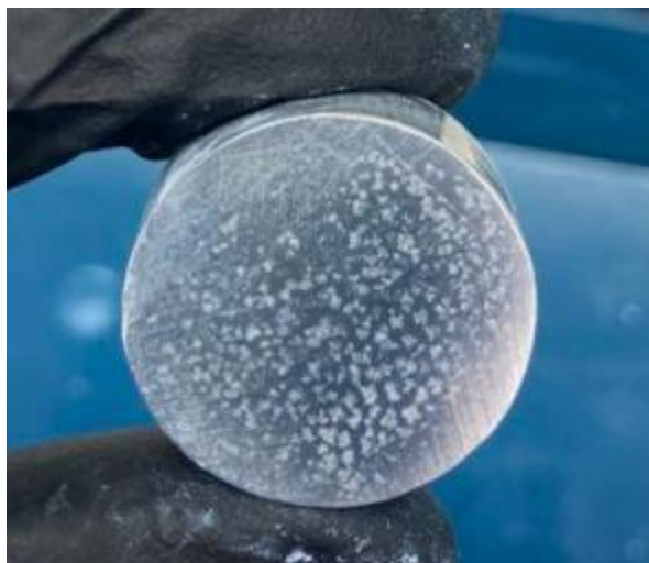
Figure 3-6. Corrosion after paint removal from an aluminum sputter coated 7075 disk.
