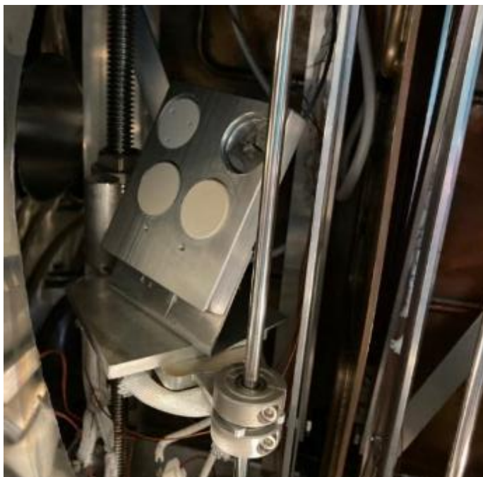
Figure E-2. Solar White coupons in sample holder after UV exposure to approximately 844 ESH NUV and 458 ESH VUV. Tile sample 21Y-131 was not present in the holder at the end of the test as it slipped out of the holder during UV-VIS-NIR measurement after the second increment and broke.
