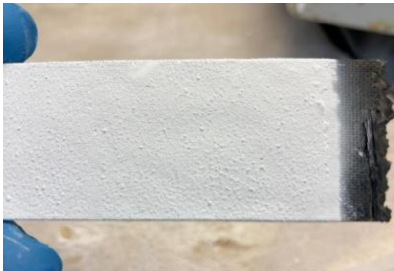
Figure 3-1. Carbon composite sample coated with 15 layers of paint.
