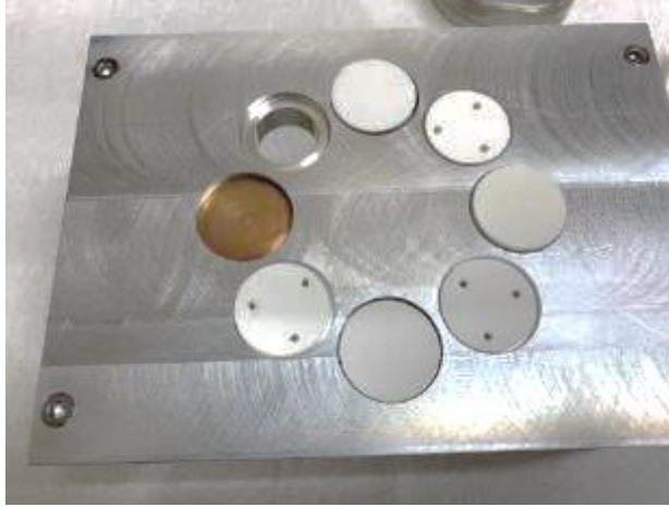
Figure D-3. Solar White coupons in sample holder after atomic oxygen exposure to a fluence of 1.31 \times 10^{21} atoms/cm 2 .
