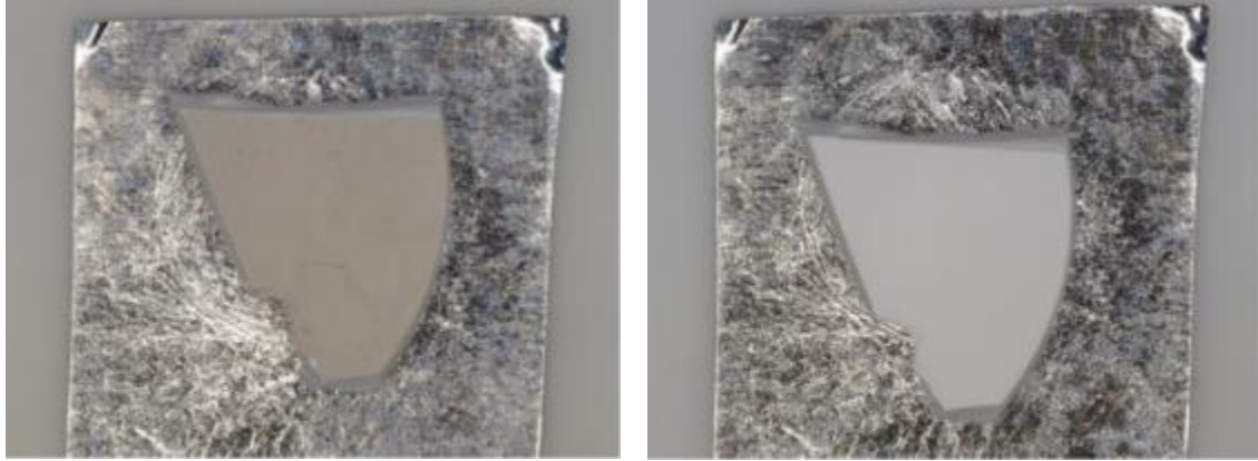
Figure 3-38. Discolored Y_2O_3 tile before (left) and after (right) heating in air.
