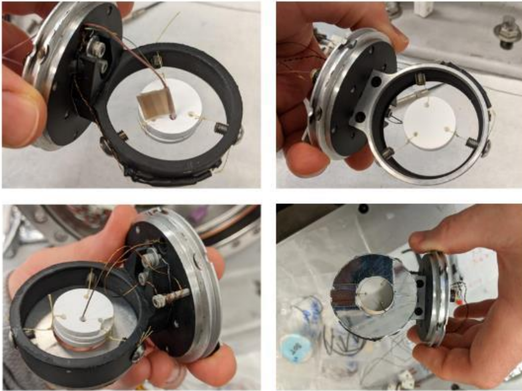
Figure C-13. Sample holder configuration comparison: no shield or wire anchor (top) vs. sample shield and wire anchor (bottom).
