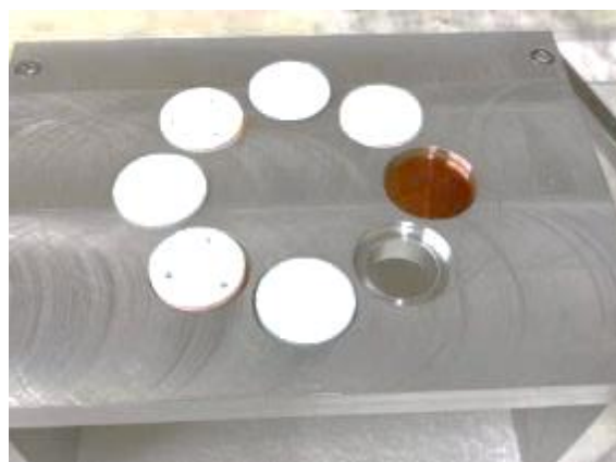
Figure D-1. Solar White samples in aluminum sample holder with Kapton fluence witness.
