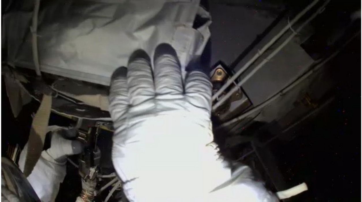
Figure 3: After routing a pair of Ethernet cables along the port truss out to the Camera Port 8 on the International Space Station, NASA astronaut Michael Hopkins leaves a bag over the end of the cable in March 2021. ( Source: NASA)
