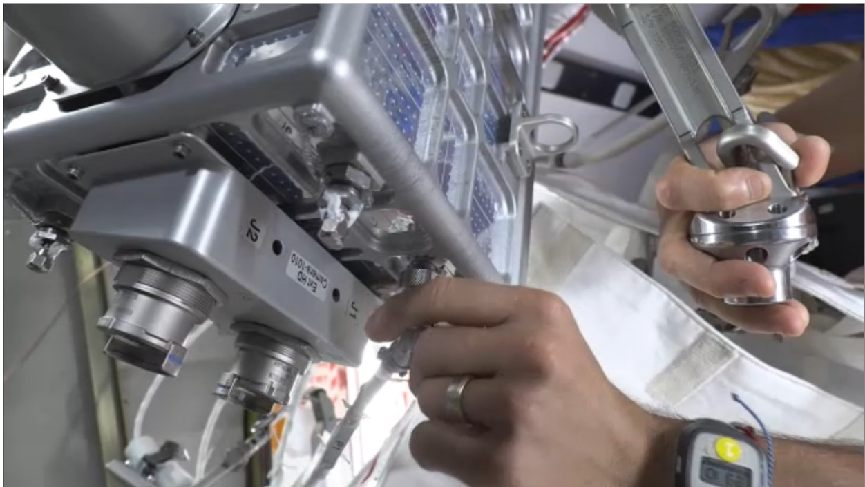
Figure 2: NASA astronaut Raja Chari double-checks the Ethernet connection to the replacement camera's test port on March 17th. (Source: NASA)
