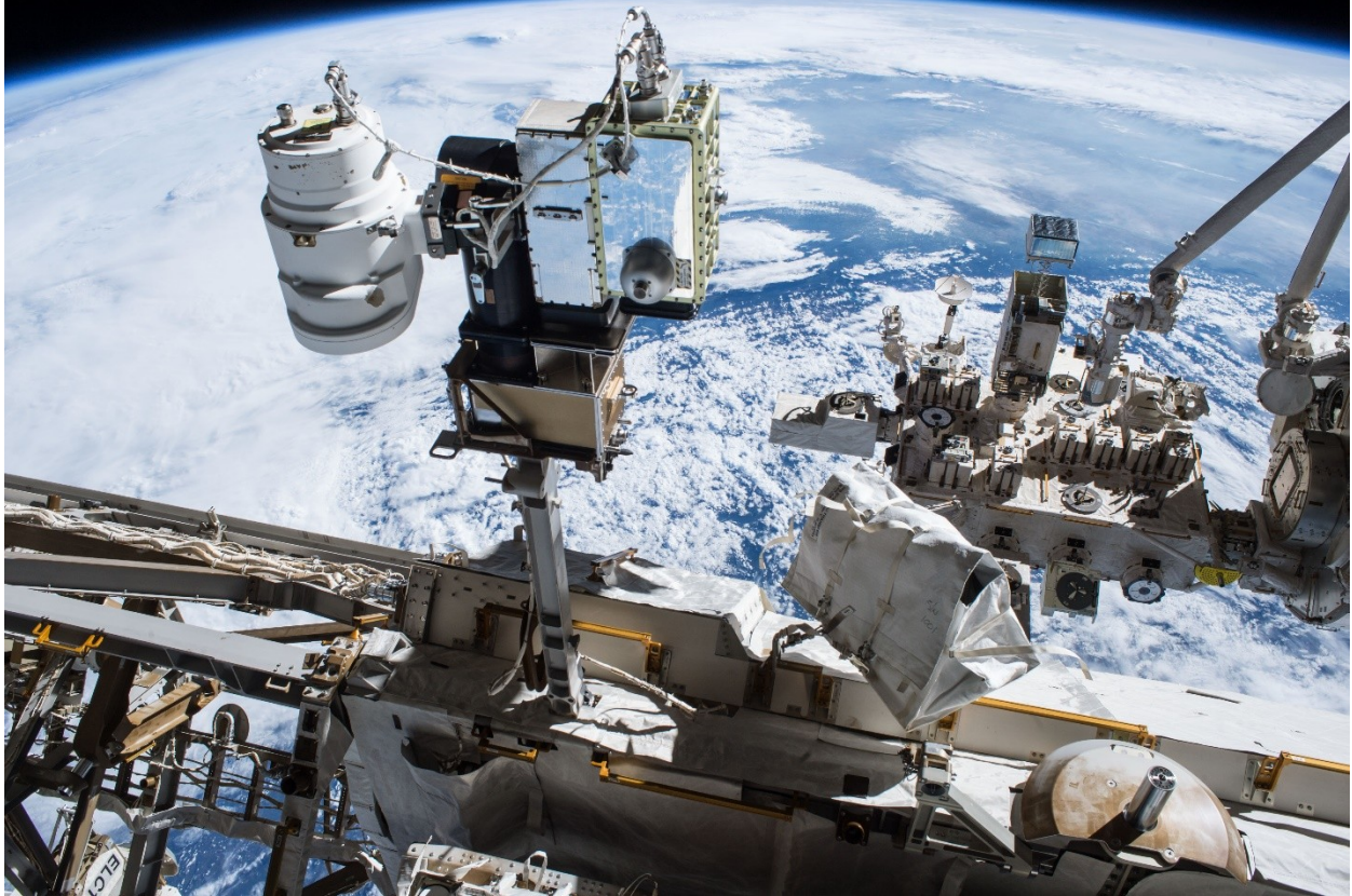
Figure 4: The External Television Camera Group (ETVCG) is comprised (left to right) of a luminaire, a motorized pan-and-tilt positioner, and standard-definition camera. In 2016, space walkers mounted a high-definition digital camera (EHDC) beside the analog camera and re-routed luminaire power to pass through the digital camera assembly. The digital camera connected wirelessly as a Wi-Fi client. Close-out photo of Camera Port 8 EHDC installation taken by astronaut Jeff Williams. (Source: NASA)
