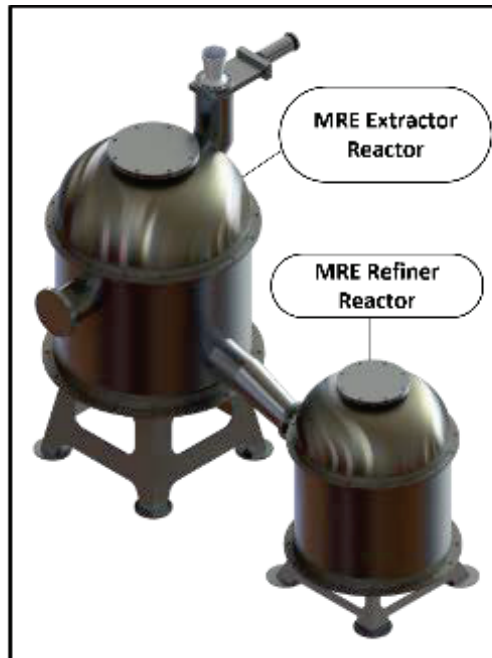
Figure 6.5.3-2. Schematic of FarView Molten Regolith Electrolysis System
