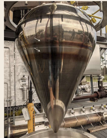
Discolored bands indicate separation and reattachment points on spike wall.
