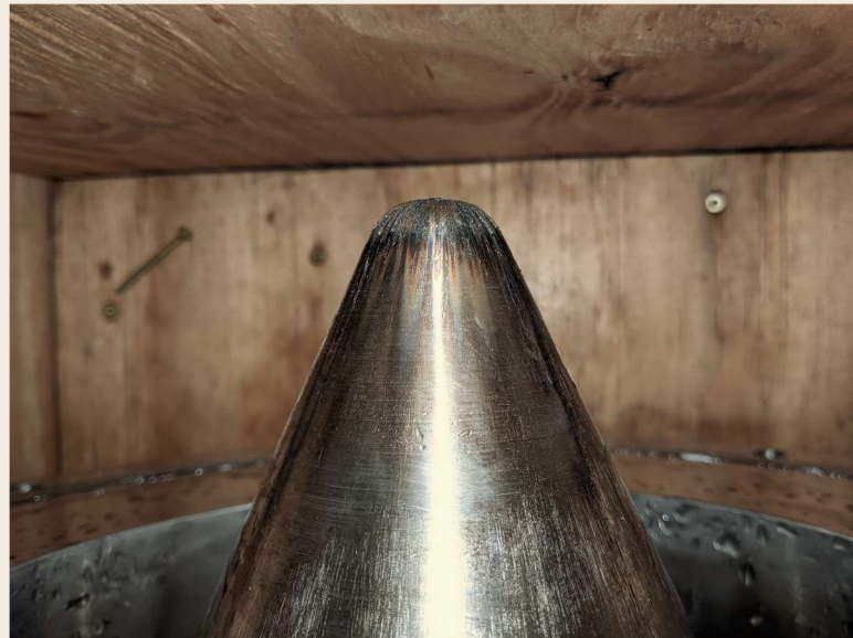
Side view of nosecone 1 erosion after 11.4 seconds of firing.
