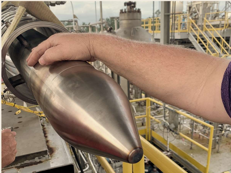
Inspection of nosecone 2 erosion after 14 seconds of firing.
