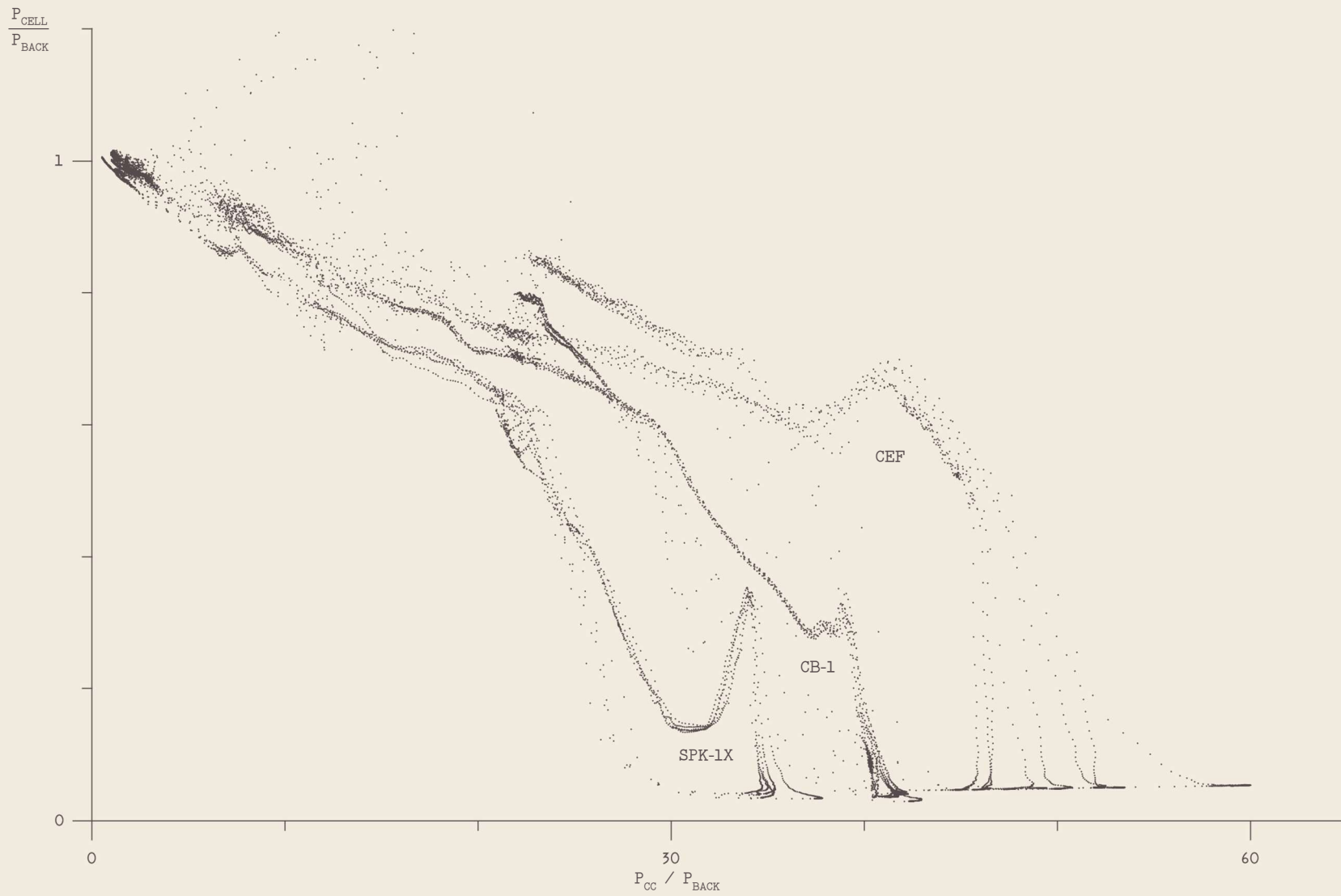
Figure 23. Pumpdown performance comparison: best-starting diffusers of each topology.
