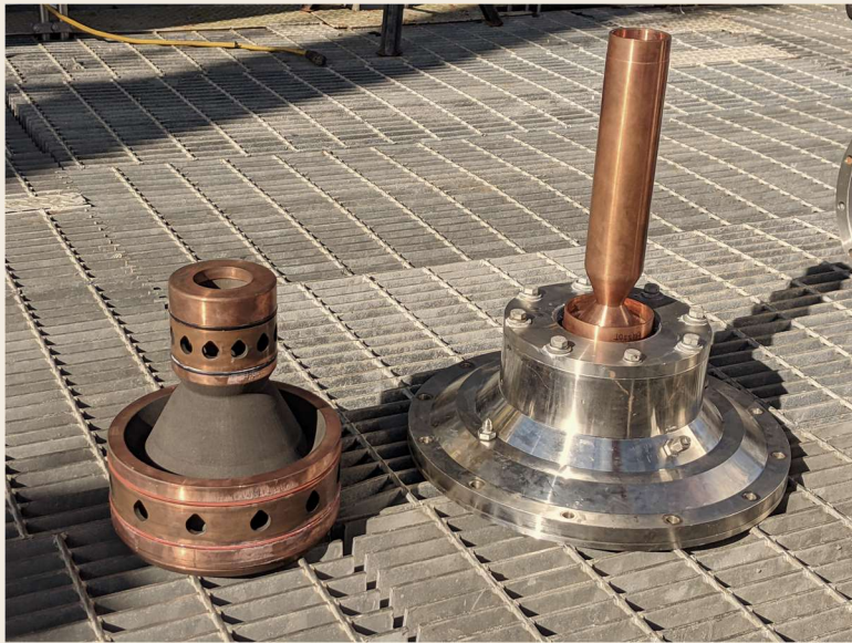
DMLS and conventionally-machined rocket liners.
