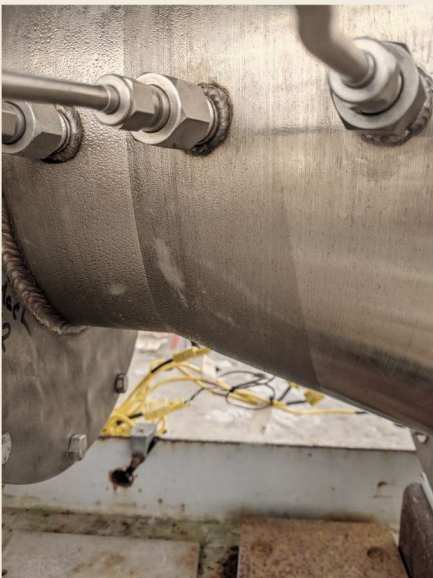
Shell-wall boundary layer separation line revealed by external condensation.
