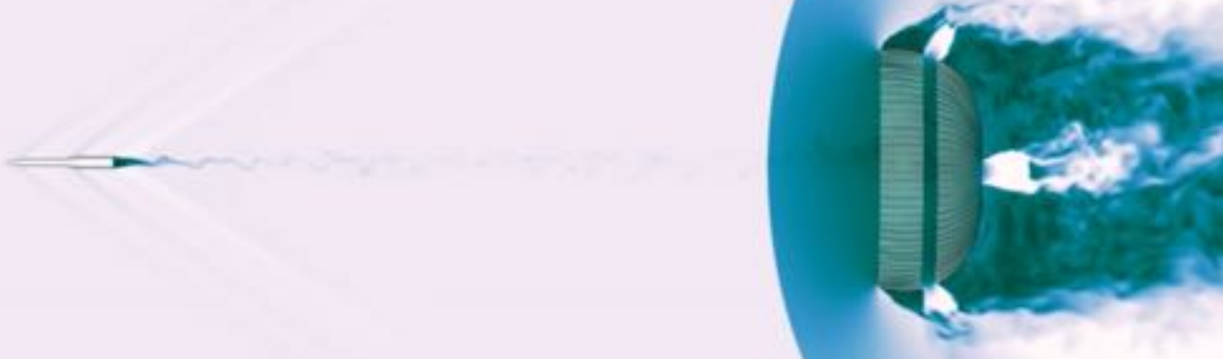
Saturated pseudocolor contours of Mach number shown on a cut-plane through the center of the domain for a medium CFD - fine CSD simulation of ASPIRE SR01.
