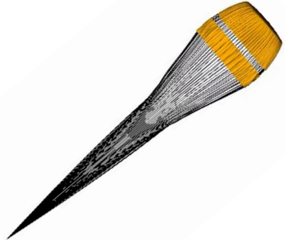
Picture showing parachute structural mesh as it is deformed by a uniform outward pressure in a structural dynamics simulation (decoupled from CFD).
