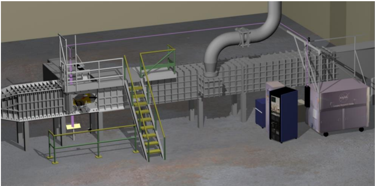
Figure 12: PLIF system in the 31-Inch Mach 10 Tunnel
