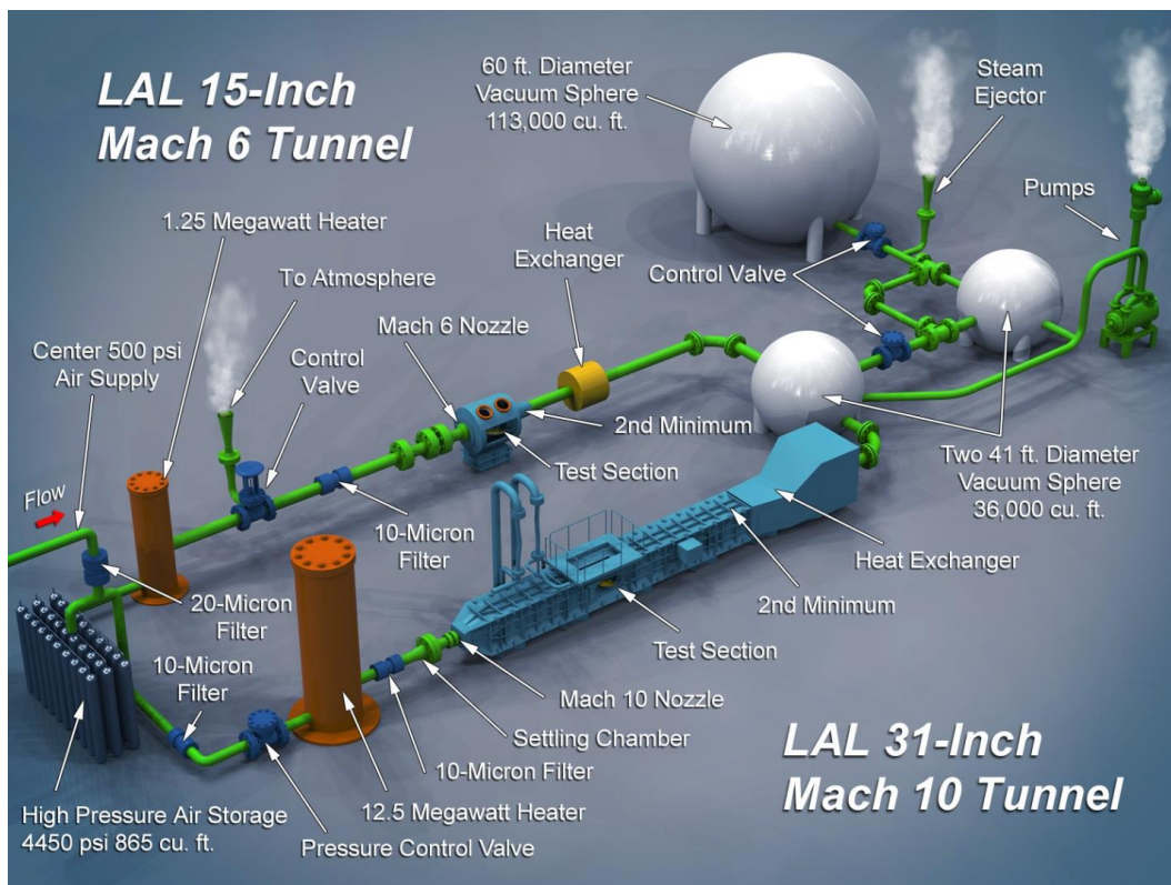
Figure 4: LAL 31-Inch Mach 10 and 15-Inch Mach 6 High Temperature Tunnels
