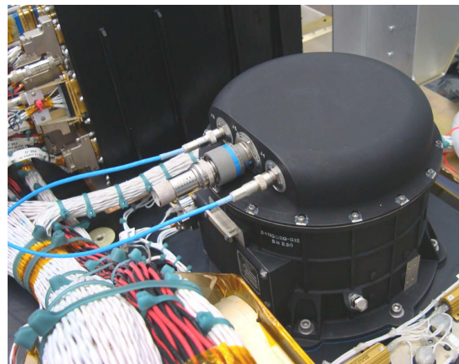
Left: MIMUs on the Mars Reconnaissance Orbiter spacecraft shown during assembly and integration. Above: Lunar Reconnaissance Orbiter MIMU sensor hardware mounted on spacecraft panel in flight configuration during pre-launch integration and test.
