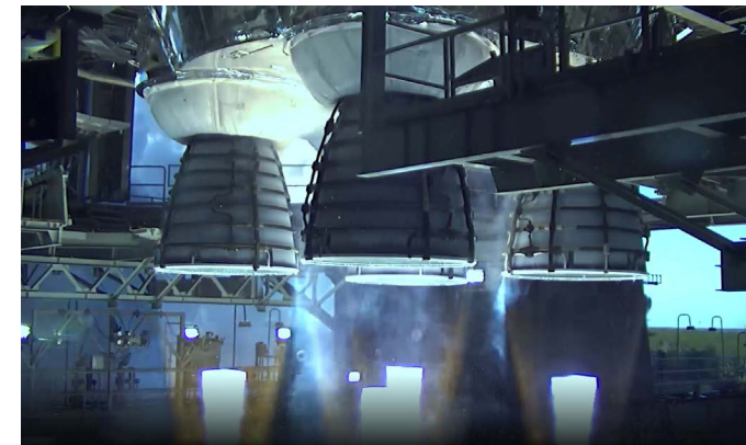
Contaminants in liquid propulsion systems must be controlled to increase operational reliability. Left: Test firing of the SLS RS-25 core stage engines. Right: SLS core stage preparation for Artemis I mission.
