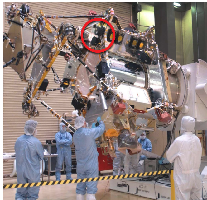
Left: MIMUs on the Mars Reconnaissance Orbiter spacecraft shown during assembly and integration. Above: Lunar Reconnaissance Orbiter MIMU sensor hardware mounted on spacecraft panel in flight configuration during pre-launch integration and test.
