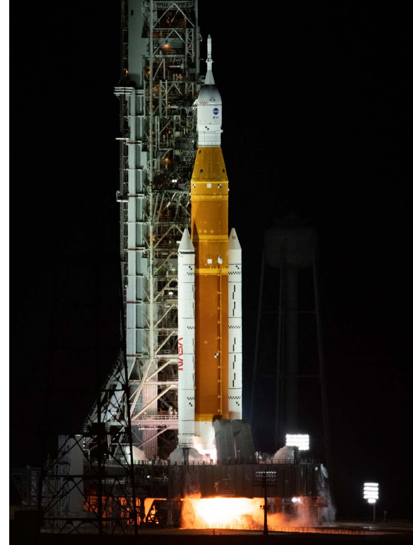
SLS is a liquid-fueled launch vehicle. Mitigation against fuel slosh instabilities is included in the flight control system.
