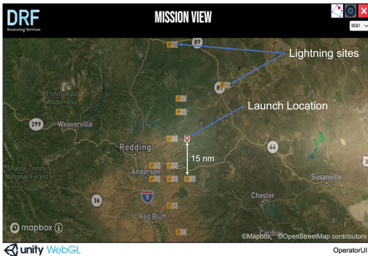
Figure 1: Mission View application displaying launch location and target lightning sites to visit with limited air-vehicle resources. The problem is to autonomously select the highest priority subset of sites, to plan a flyable vehicle trajectory to visit them with limited control authority, and to estimate remaining battery charge.
