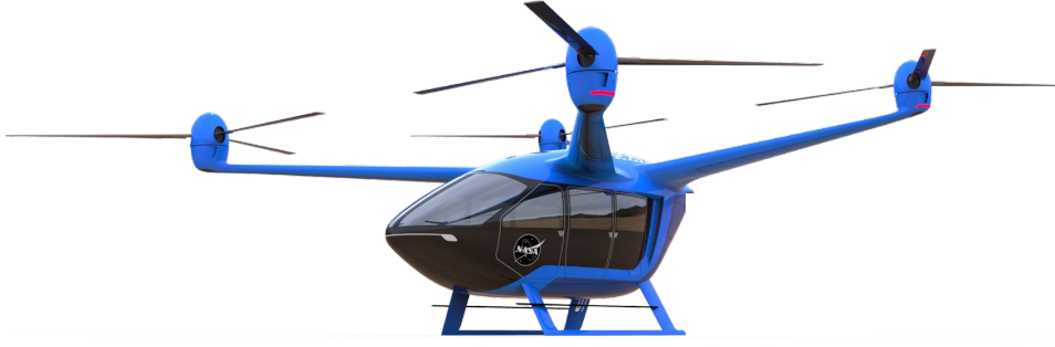
Figure 2: Selected 1200-lb payload quad eVTOL concept vehicle.
