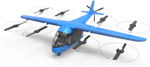
Fig. 1 Rendering of a Lift+Cruise NASA reference configuration.
