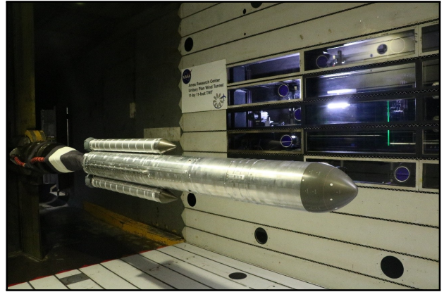
(b) SLS Block 1B Cargo 2.5%-scale RBM tested during the ARC UPWT ATAT. [Photo: NASA]
