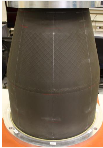
Figure 5. Test article potted in the end rings.
