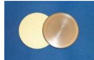
Ceramic Thermocouple fabricated at University of Rhode Island
