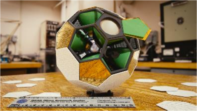
Concept illustration of the CFIDS detector assembly (cables, electronics not shown)
