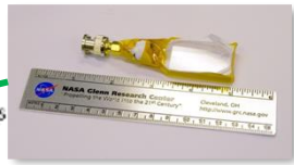
GaP Diode for Solid-State Trigger/Veto Detectors (U.S. Patent 10,429,521)
