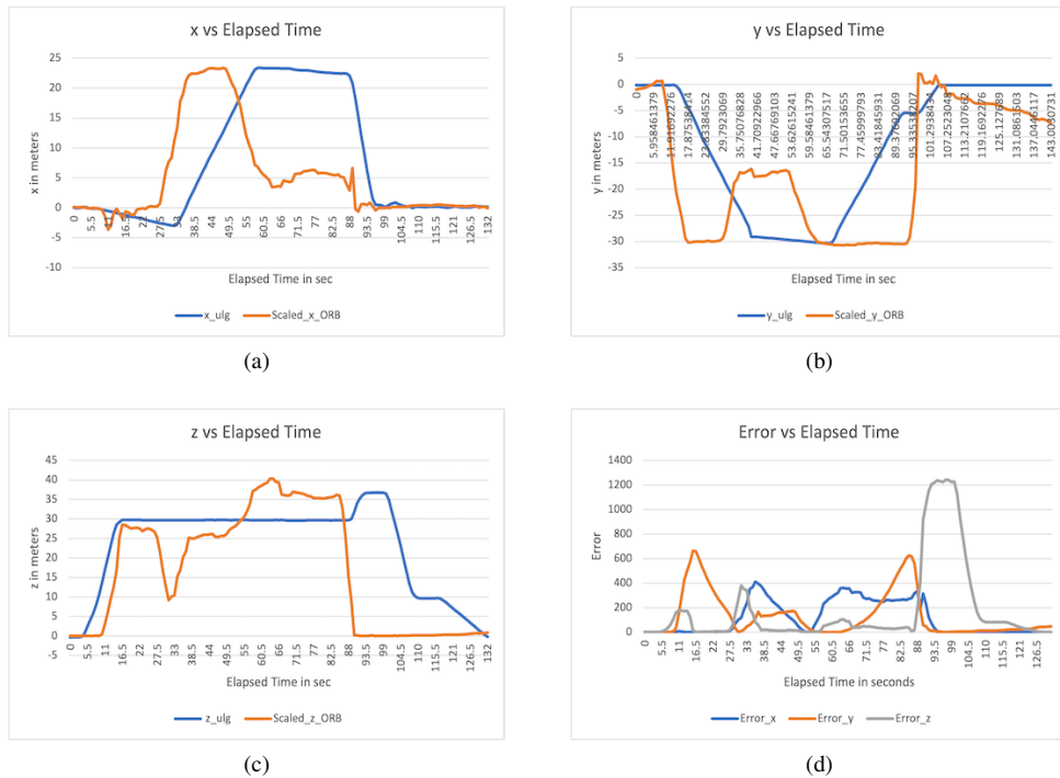
Fig. 6 x, y, z and the error versus the elapsed time plot for DART_SQ ORB-SLAM2 outputs
