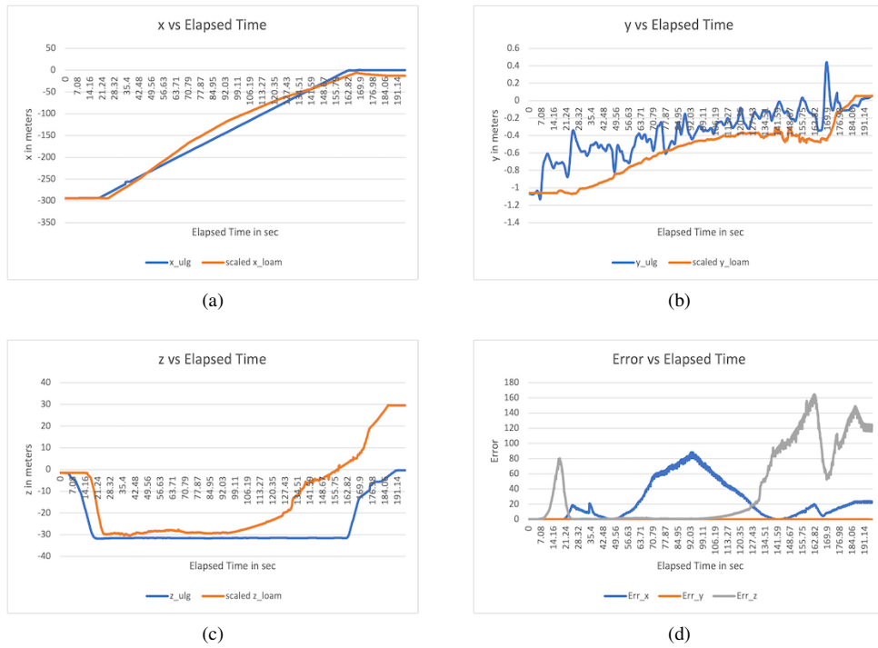
Fig. 3 x, y, z and the error versus the elapsed time plot for DFM_2 A-LOAM outputs
