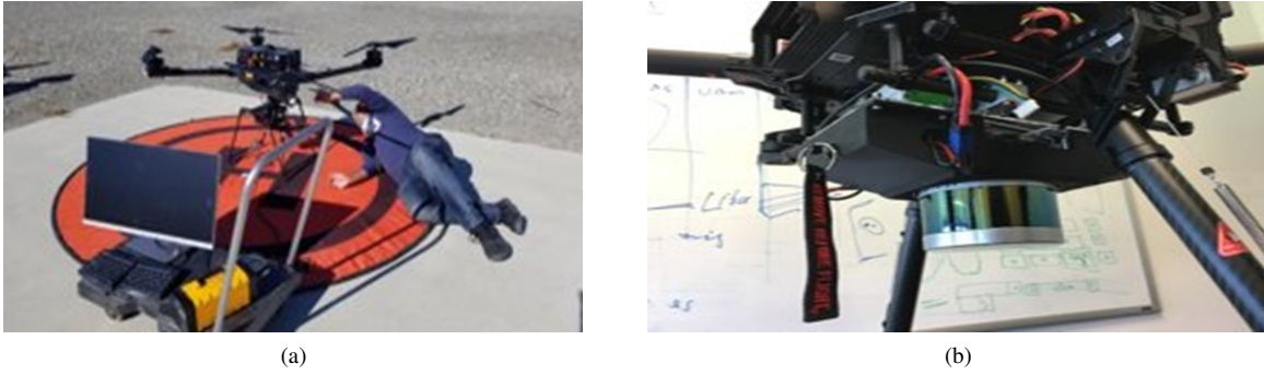
Fig. 5 ARC flight images (a) The flight in its landing/takeoff pad with the team calibrating (b) The payload with the sensors and the NUC i7 CPU
