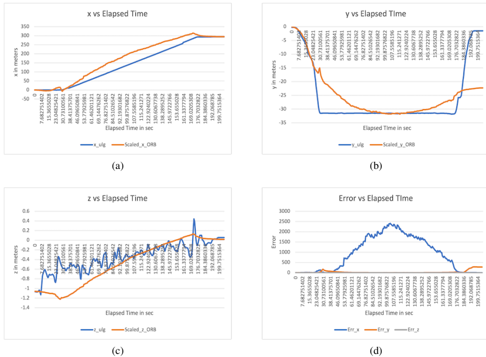
Fig. 8 x, y, z and the error versus the elapsed time plot for DFM_1 ORB-SLAM2 outputs
