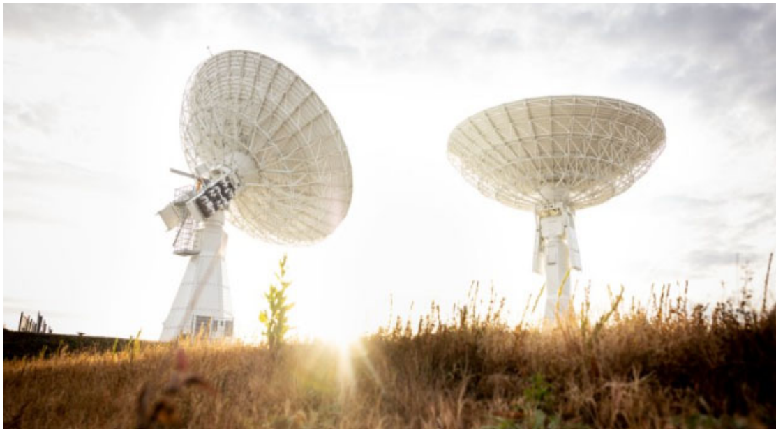
Figure 11.24: Viasat’s new Large-Aperture Space-to-Ground Communication Antennas ready to support Lunar, Cislunar, Deep Space and DoD Missions. Credit: Viasat.
