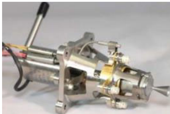
Figure 4.6: GR1 thruster. Credit: Aerojet.
