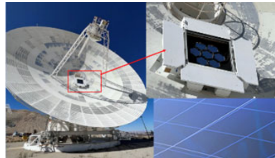
Figure 11.35: JPL's DSS-13, a 34m RF antenna, showing a 1.3-meter optical aperture in its center. Credit: NASA JPL.
