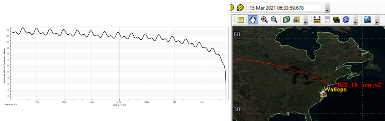
Figure 13.9: Targeting of the TES-10 Exo-brake is achieved by modifying the drag area of the modulating Exo-brake. (Left) The plot includes actual GPS readings and the approximate ballistic coefficient achieved at different parts of the mission. (Right) The simulated reentry location of TES-10. The spacecraft overshot but still demonstrated the capability to target a particular location by modifying its ballistic coefficient. Credits: Jose Alvarellos et al. 2021/Sanny Omar/NASA.
