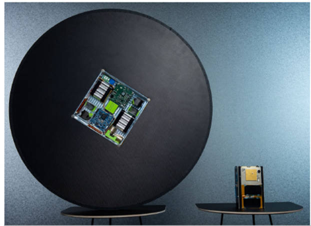
Figure 6.5: Comparison of DiskSat structure to a 2U CubeSat structure. Courtesy of and reprinted by permission of The Aerospace Corporation.
