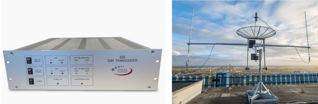
Figure 11.21: (left) ISIS ground station hardware, transceiver rack and tracking antenna (right). Credit: ISPSPACE.
