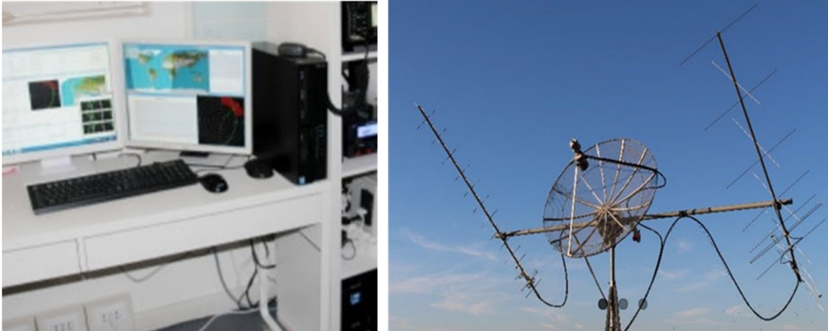
Figure 11.20: (left) GAUSS ground station hardware, transceiver and (right) tracking antenna. Credit: GAUSS Srl.
