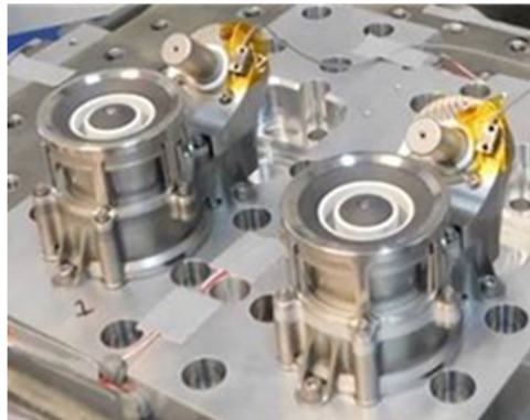
Figure 4.41: Two flight Aurora HETs undergoing qualification testing. Credit: Orbion Space Technology.
