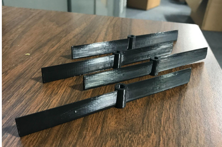
Figure 24: NACA 0015 3D Printed Propellers
