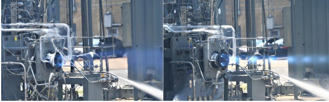
Fig 9. Example of a typical throttled test where valves are toggled to yield a lower (left) and higher (right) power condition.
