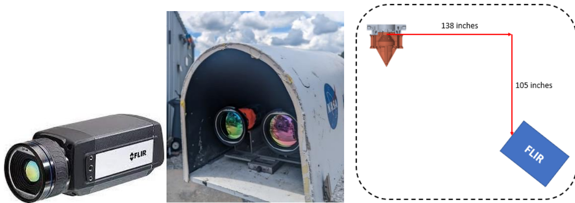
Fig 10. FLIR A655 body (top left) and dual imager setup with FOL89 7-degree lenses (top right), and diagram of FLIR placement (bottom).
