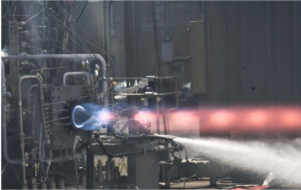
Fig 21. High power liquid/liquid direct injection at MR 3.47 and estimated mean pressure of 330 psia.
