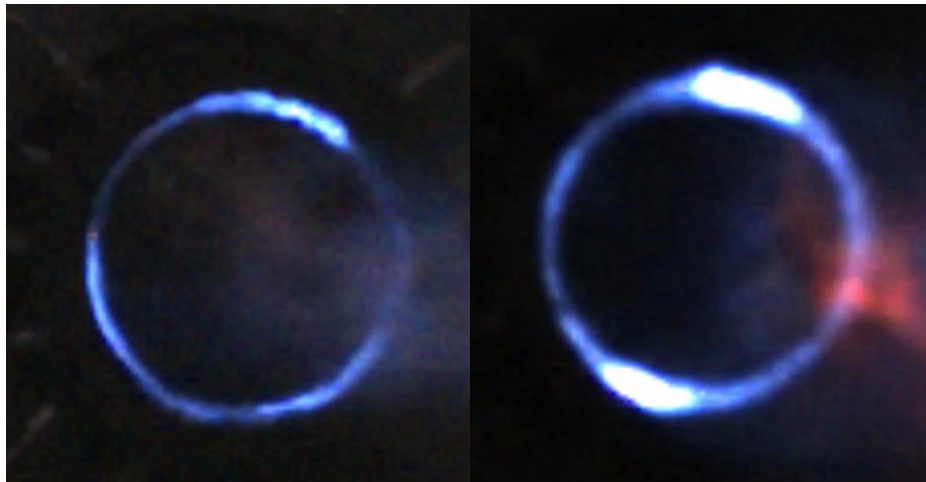
Fig 31. 3-wave (left) and 2-wave (right) corotating modes observed in test 026 and 028, respectively.
