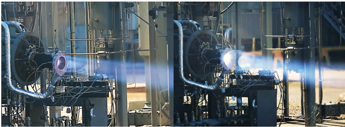
Fig 28. LLAMA lander engine throttle test from mean chamber pressures of 130 psia (left) to 350 psia (right) with LOX/CH 4 .
