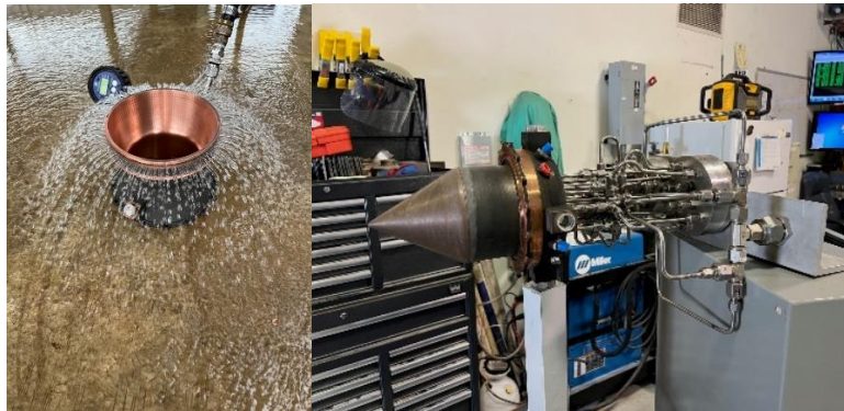
Fig 5. Channel flow testing (left) and buildup of hardware assemblies (right).
