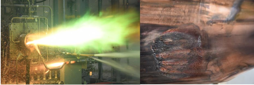
Fig 13. Hot fire burn-through of the V2 inner body.
