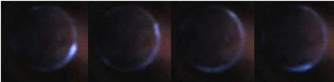
Fig 14. LOX/GH 2 3 corotating wave modes at mean chamber pressure of ~15 psig and MR = ~15.
