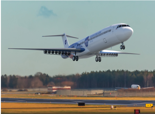
(a) SUSAN Electrofan concept during takeoff.
