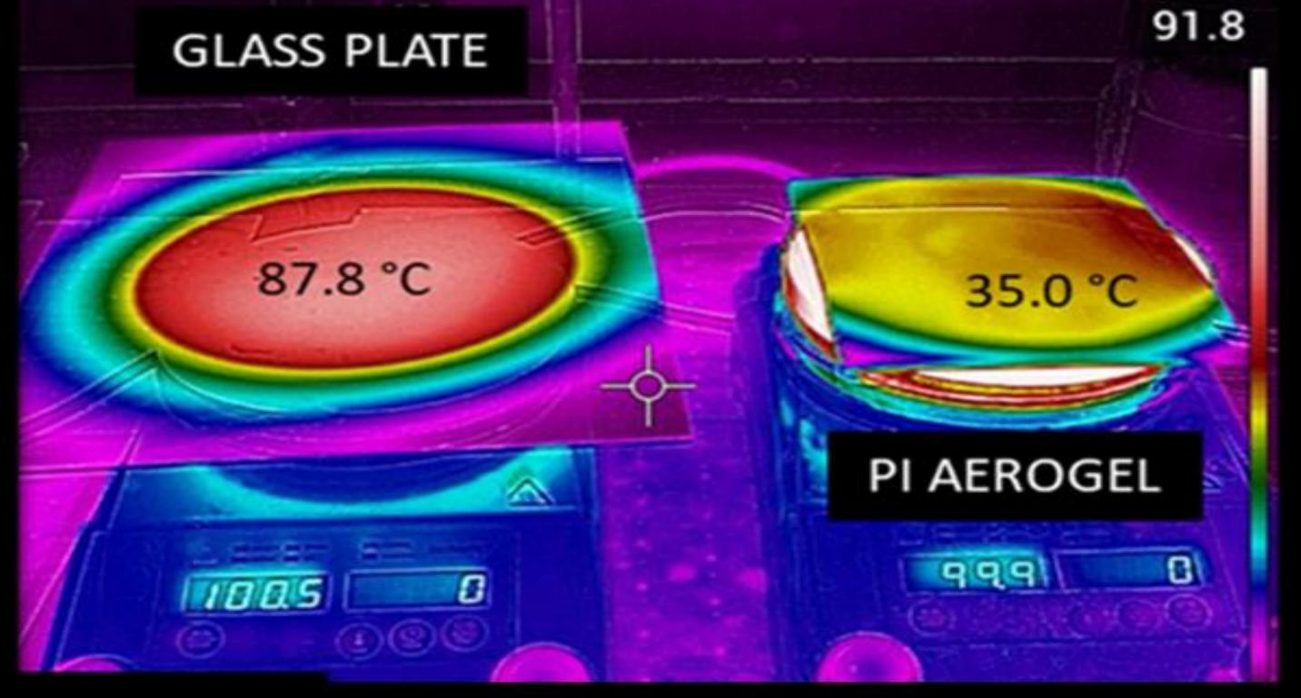
PI aerogel is 30-60 times more thermally insulating than glass at RT and ambient pressure
