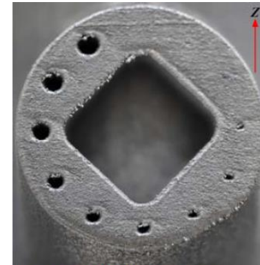
Fig. 7.20 Hole shape vs size, diamond slot, and surface roughness vs angle in L-PBF-built AISi10Mg.
