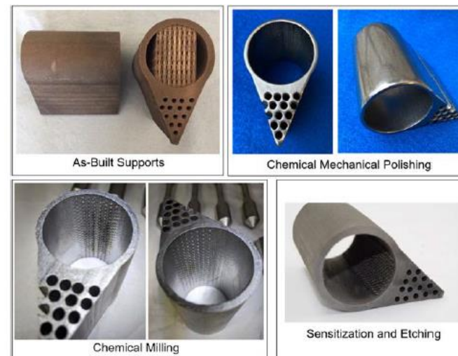
Fig. 5.20 Different chemical support removal methods for original unaltered supports from the L-PBF process. (Source: NASA.)
