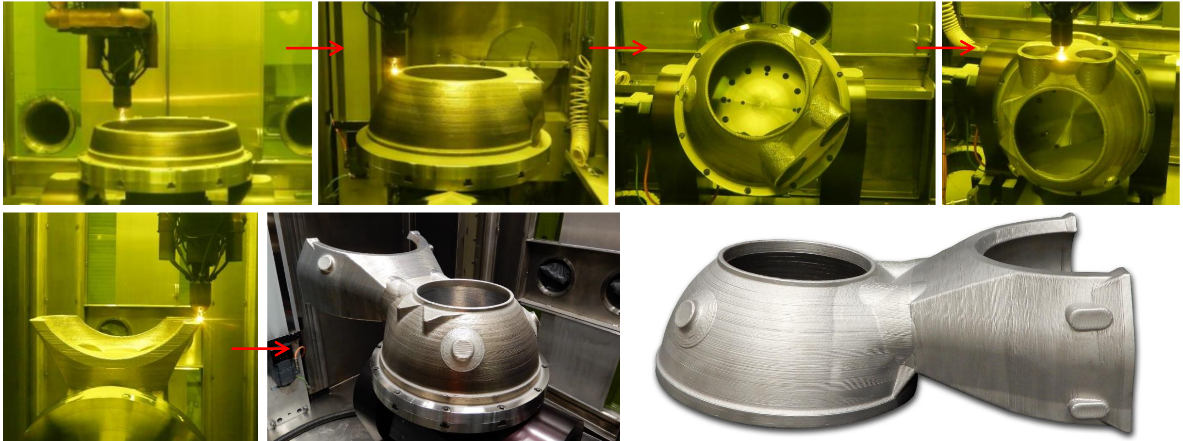
RS25 Powerhead demonstrator using LP-DED under NASA SLS Artemis Program (NASA/RPMI)
