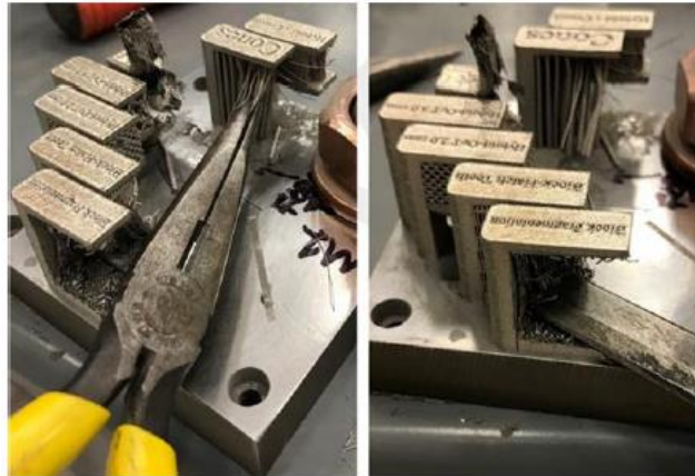
Fig. 5.13 Manual support removal using hand tools. (Source: NASA.)
