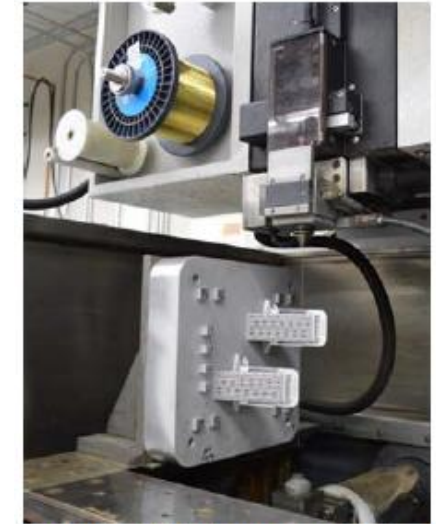
Fig. 5.23 L-PBF aluminum part fixtured wire-EDM cut chamber before the removal of specimens. (Source: Quadrus Advanced Manufacturing.)
