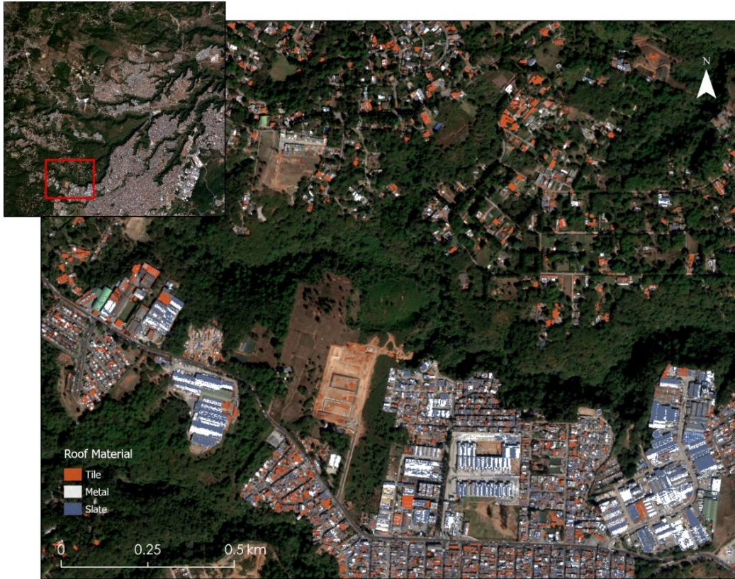
Figure 4. Zoomed in roof material classification over Basemap Satellite imagery of Guatemala City. Basemap: Esri, Maxar
