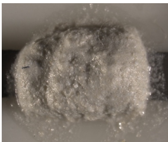
Figure 20. Epoxy sample with material fired at 1,250 °C.
