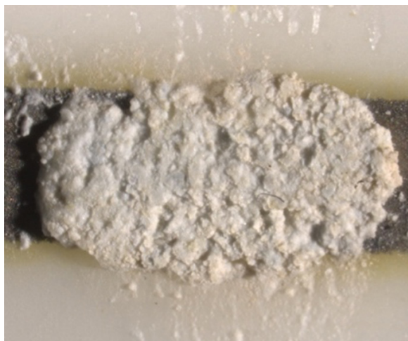
Figure 18. Epoxy sample with material fired at 1,150 °C.
