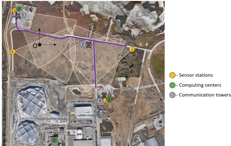
Fig. 1 Target's flight path, Sensor stations, Computing canter and Communication towers.
