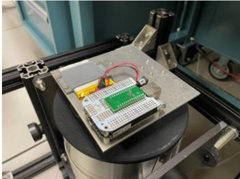
Single-axis shake table for short and long duration IMU testing.
