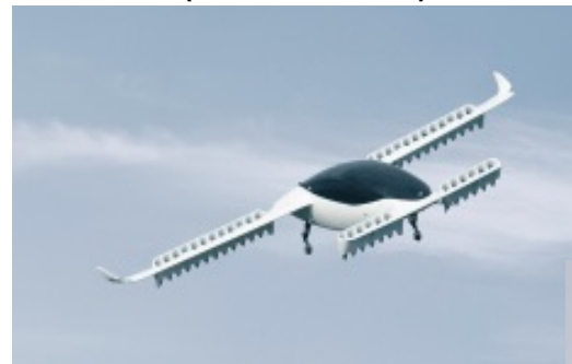
Lilium Jet (Tilt Ducted Electric Fans) [Vectored Thrust]
