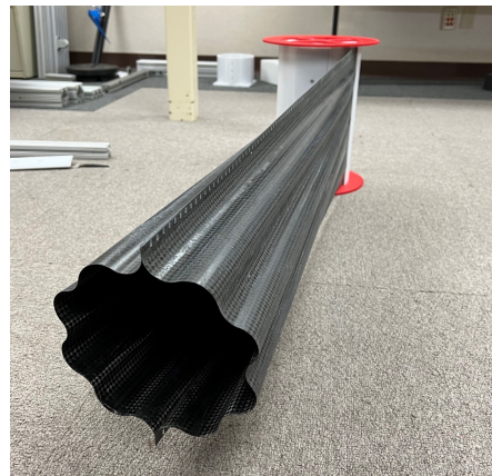
COROTUB cross-section developing from spool
