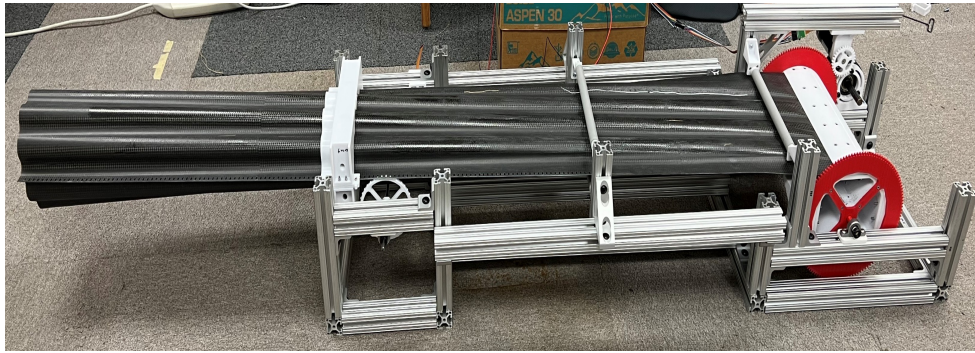
COROTUB deployment mechanism
