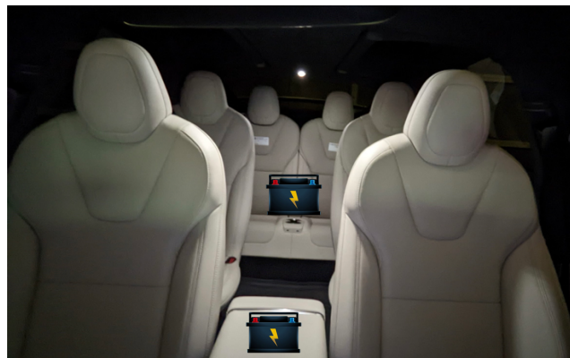
Fig. 2 A potential design to embed the spare and swappable batteries in the cabin.
