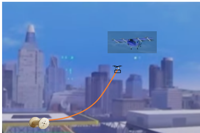
Fig. 4 A power cable being flown to charge an AAM vehicle.
