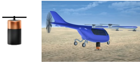
Fig. 3 A battery with rotor(s) (left) and a battery docked to an AAM vehicle (right).
