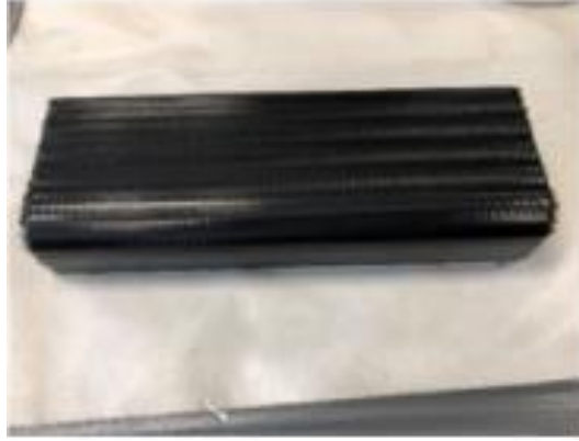
Figure 1. Cured part of C-shaped composite panel [5] (Courtesy: NASA/TM-2019-220350).
