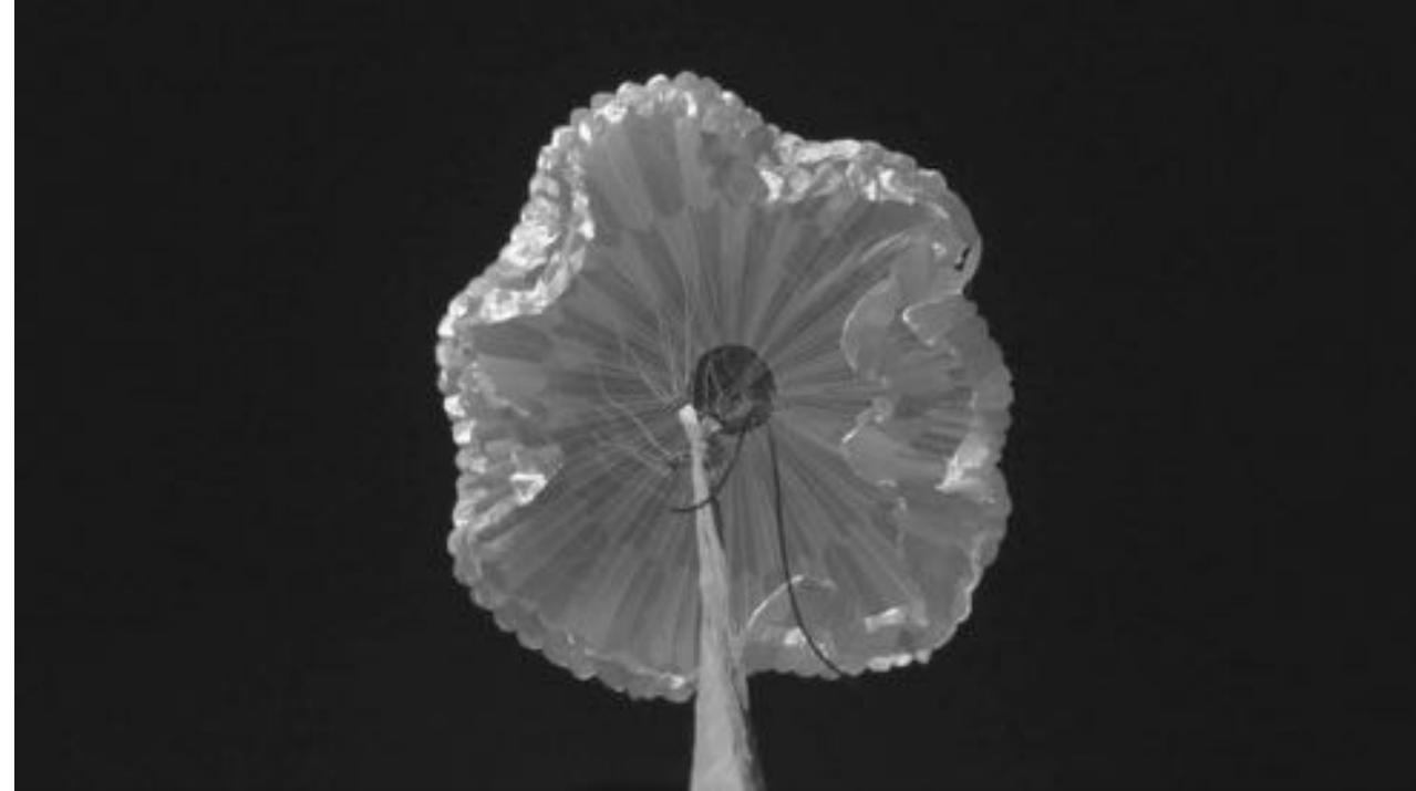
This high-definition image was taken on Sept. 7, 2018, during the third and final test flight of the ASPIRE payload. It was the fastest inflation of this size parachute in history and created a peak load of almost 70,000 pounds of force. **Credits: NASA/JPL-Caltech**
