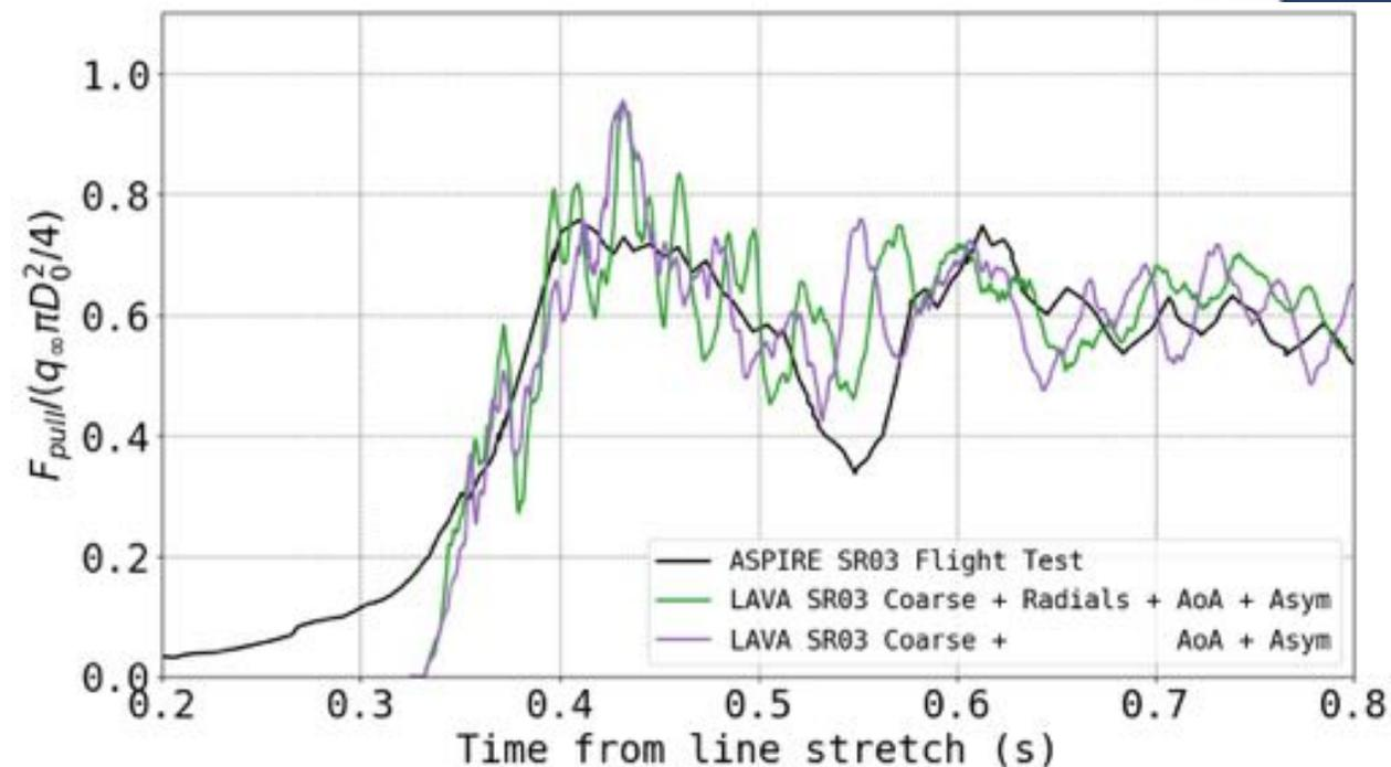
Relaxing assumption that radials act like suspension lines further damps high frequency oscillations by breaking up the possibility of standing waves, but produces very similar results.
