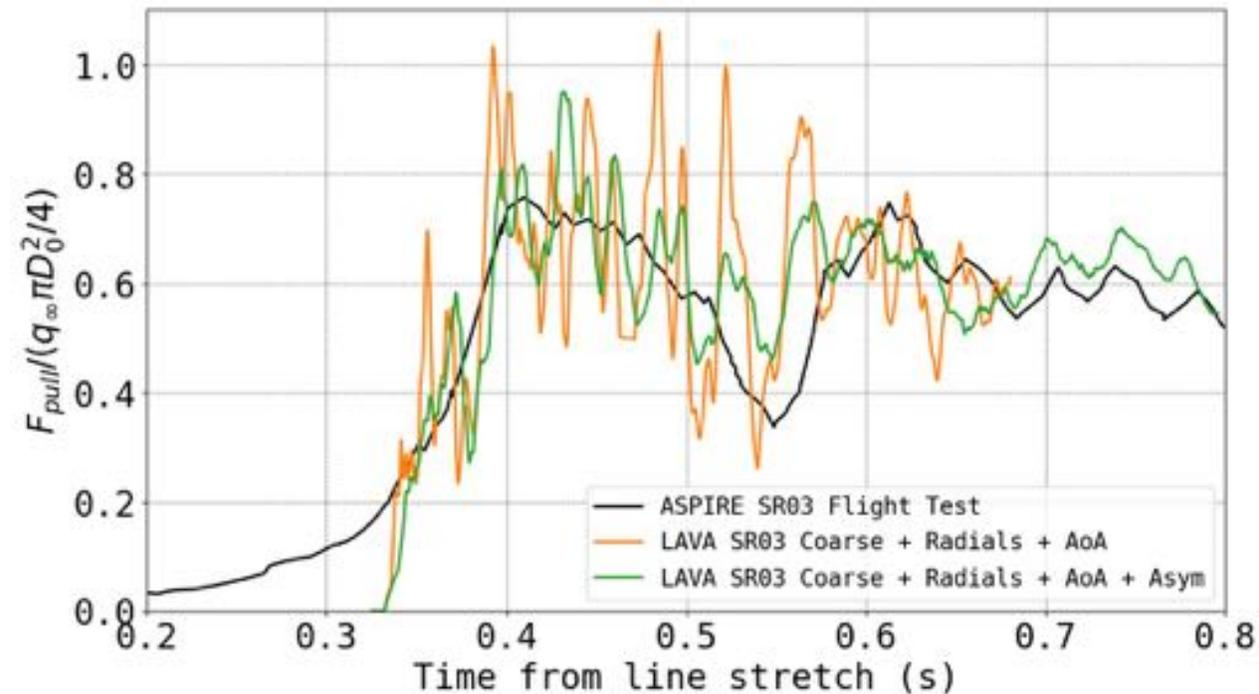
Adding asymmetry to initial parachute shape adds varying amount of slack to lines, causes uneven inflation process, and thus reduces amplitude of high-frequency oscillations caused by synchronized tension waves across radials and suspension lines.
