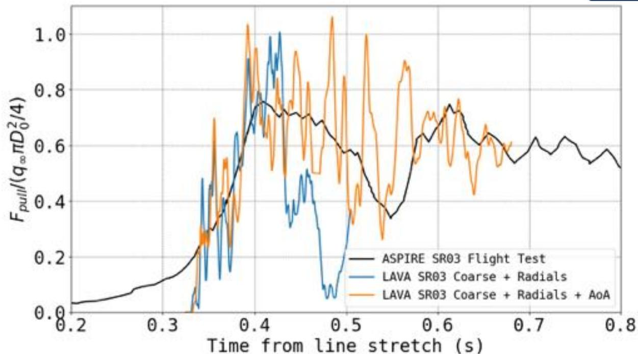
Dip down to almost zero pull force caused by quasi-2D wake bow shock interaction disappears with AoA which causes wake to break down to turbulence and bow shock to remain much flatter
