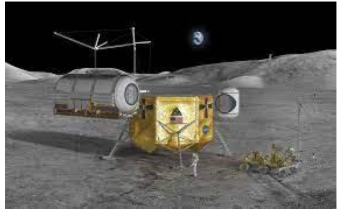
Figure 11. Illustration of Heavy LSMS Unloading a Habitat Module from a Lander
