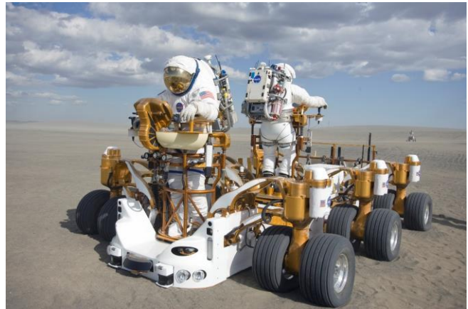
Figure 6. First Generation Chariot Prototype Configured as an Unpressurized Rover
