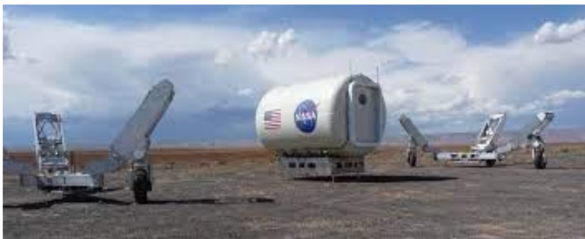
Figure 9. ATHLETE Separating into its Two Halves
