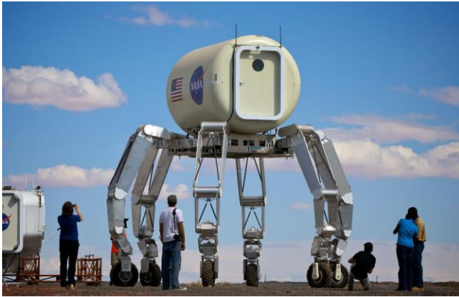
Figure 8. Half-Scale ATHLETE Prototype Carrying Mockup Habitat Module
