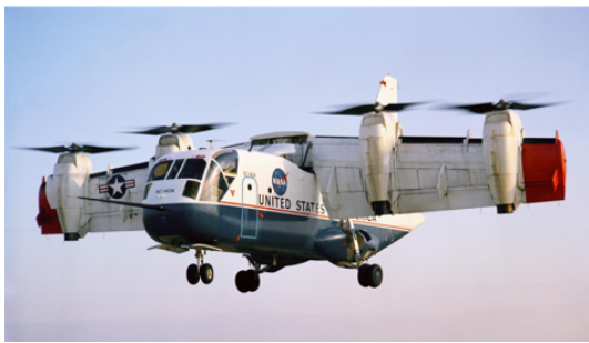
(a) LTV XC-142A tiltwing aircraft, a design featuring 4 rotors.
