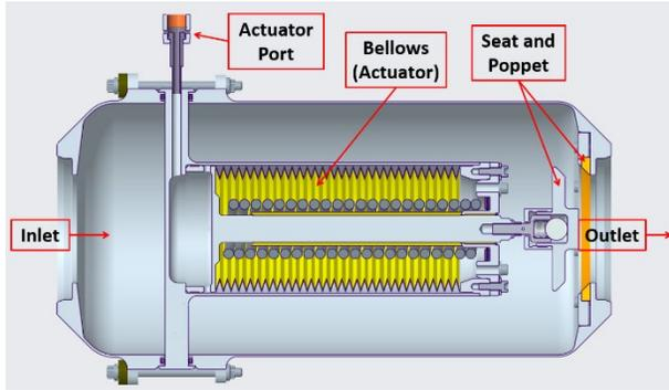
**Fig. 7 Cross-Section of LLIV Model**
