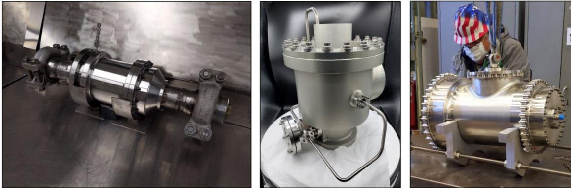
**Fig. 4 Low Leakage Test Valves: LLIV (Left), LLRV (Center), LPV (Right)**
