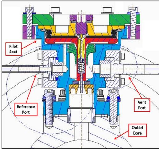
**Fig. 11 LLRV Pilot Valve Cross-Section**
