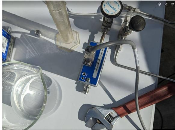
**Fig. 20 Split Configuration for Flowmeter**
