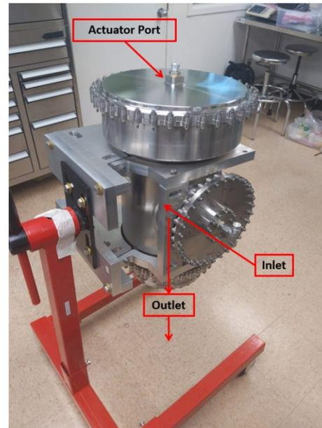
**Fig. 17 LPV in Assembly Stand**
