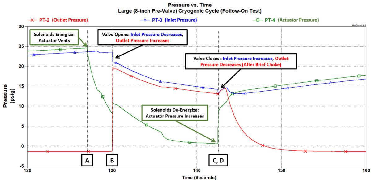
**Fig. 18 Pressure Levels During an LPV Cycle**
