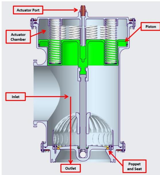
**Fig. 16 Cross-Section of LPV Model**
