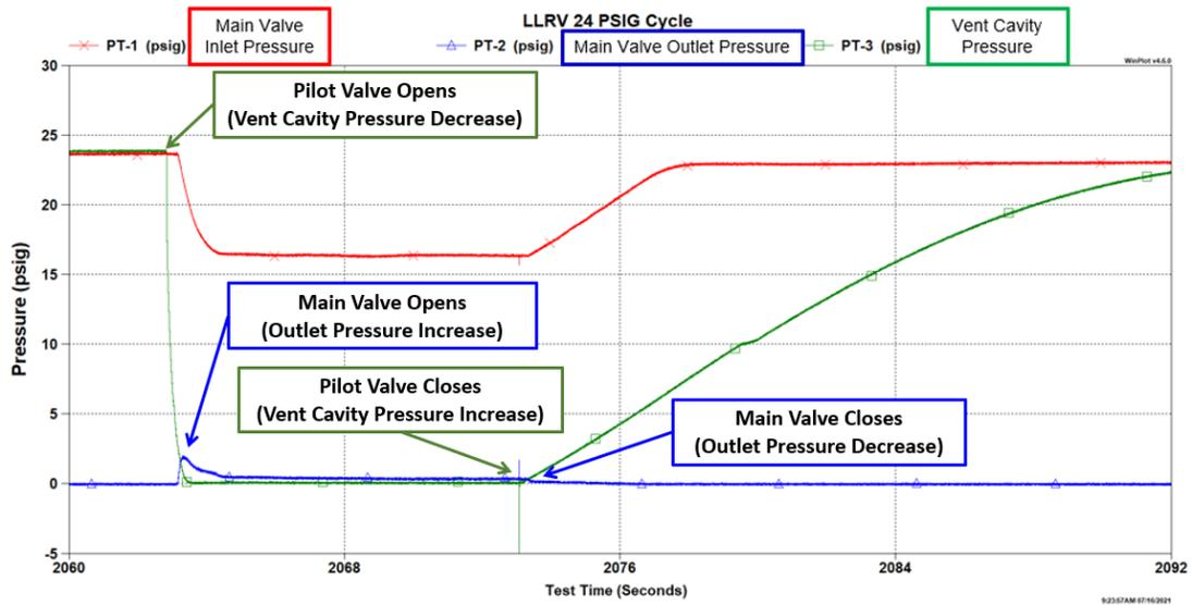
**Fig. 13 Pressure Levels During an LLRV Cycle**
