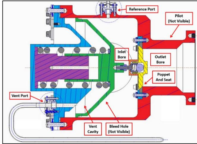
**Fig. 12 LLRV Main Valve Cross-Section**
