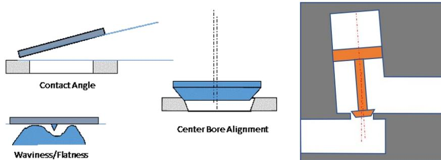
**Fig. 2 Imperfections and Misalignments Between Sealing Surfaces**
