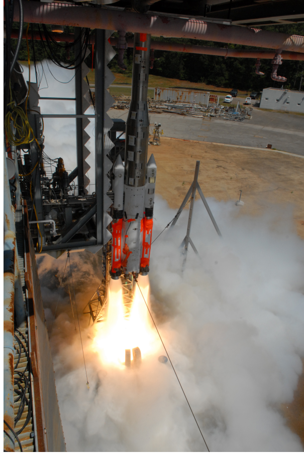
Fig. 3 Photograph of the SLS Scale Model Acoustic Test (SMAT) during an elevated vehicle case meant to model vehicle lift-off [25].
