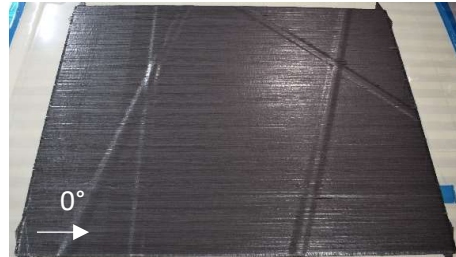
d) Activity 5h – thin ply for all stiffeners.
