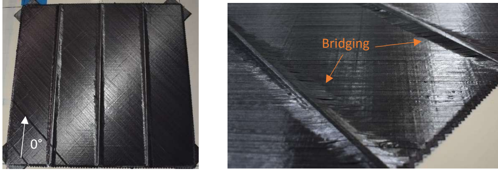
Figure 4. Skin ply interleaved every third stiffener ply showing full panel and close-up.
