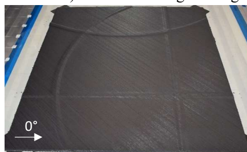
d) 5d: 76.3-cm-radius arced stiffeners.
