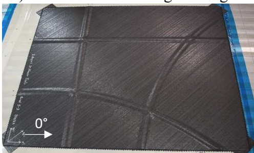
c) 5c: 114.3-cm-radius arced stiffeners.
