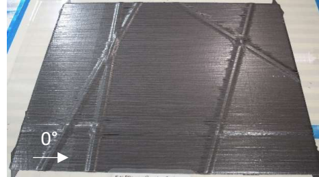
b) Activity 5f – thin ply off-axis angled skin plies.
