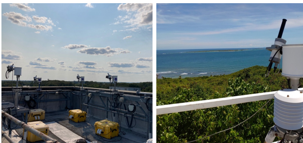
Figure 4.6.2: Left, instruments on the B33 roof are tested after laboratory calibrations. Instruments are sent to collaborators, for example Pan60 in Fajardo, Puerto Rico operated by PI Olga Mayol (right).
