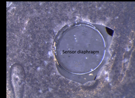
Optical Images Of Resistive Pressure Sensor Face After GEER Testing: Structure Maintains Integrity
