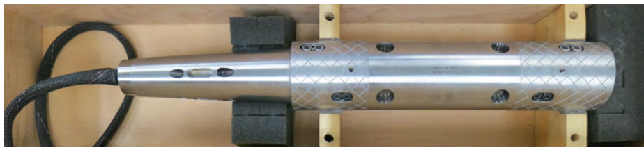
Fig. 1 Basic layout of NASA’s 2.5 inch MK40B force balance.
