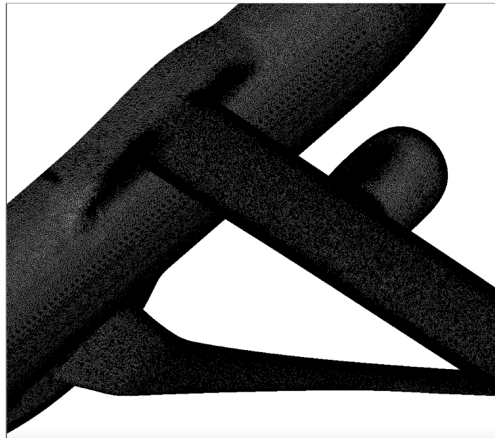
Figure 11 Close View of Mach 0.8 TTBW CFD Mesh
