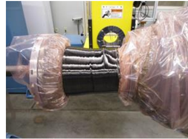
Figure 16 C. High Tension Dry Overwrap
