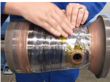
Figure 8 A. Shrink Tape Application
