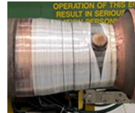
Figure 10 C. Fiberglass High Tension Overwrap
