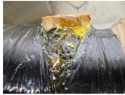
Figure 6 C. Wrinkling in Prepreg
