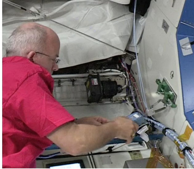
Fig. 6 Astronaut Jeff Williams Performing the First In-Space Experiments with Gecko Grippers
