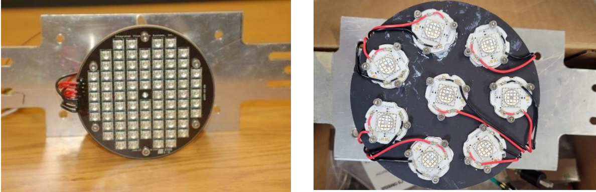
Fig. 21 (left) older version of LED lighting for NTF from Ref. 14 employing 80 LED dyes; (right) newest version of LED lighting employing 8 LED dies.
