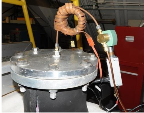
Fig. 3 Air insertion line showing heating tape (to keep air from freezing upon injection) and solenoid for remote operation.
