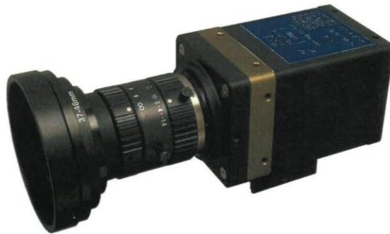
Fig. 5 Photograph of the PSP-CCD-M Interline transfer CCD camera.
