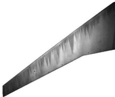
Fig. 26 Slow-roll cryogenic PSP image showing permanent turbulent wedges
