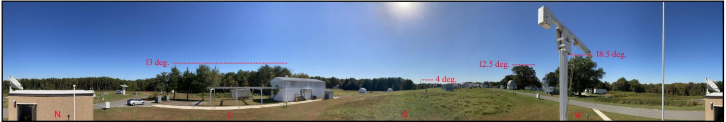
Figure 3. LCOT @ GGAO : RTA Horizon Scan shows mostly unobstructed elevations above 13deg over 360deg azimuths.
