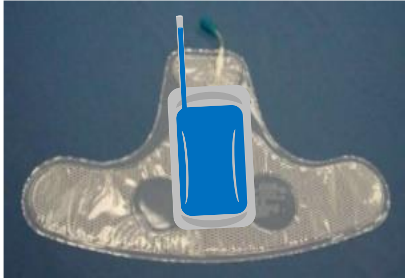
Figure 2. Rough concept of a liquid filled bag on top of an empty disposable in-suit drink bag.
