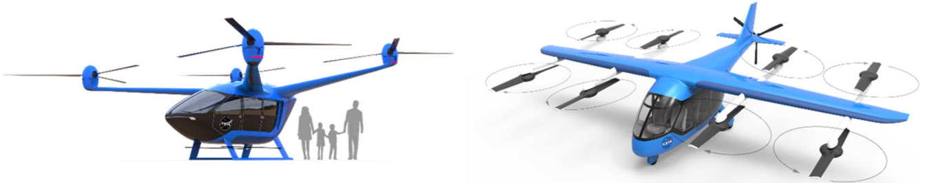
Fig. 1 NASA RVLT reference vehicle configurations considered in this study: quadrotor (left) and lift plus cruise (right).
