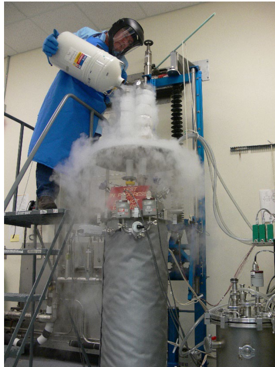
Figure 1. Filling Cryostat-100 with LN 2 in Preparation for Insulation Testing Image Credit: NASA
