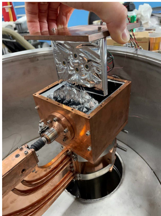
Figure 2. Space Irradiance Simulator 8 Test Setup Powered by a Cryomech AL230 G-M Cryocooler Image Credit: NASA
