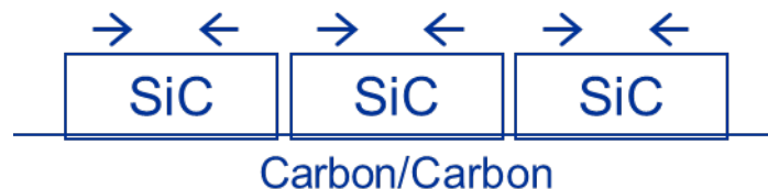
SiC crack mouth 1200°C/0.5 hr/air
